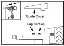
Figure 5. Removing guide cover.
